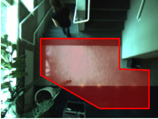
Figure 3: Example of the annotation of the ground plane, used to compute the prior probability that a person can be located at any particular position in the image. Similar regions were annotated for all three cameras.
